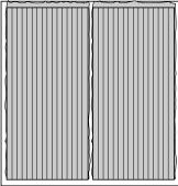
Figure 19 - Correct Burner Flame Pattern (Model VP11 Shown)
